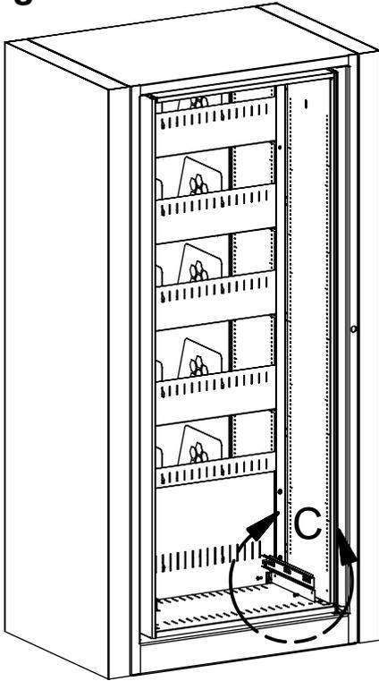
**Step 2:** Attach each Bracket with Large Part of Slide to desired location on cabinet with two #10-24 x 1/2" Type 'F' Phillips Pan Head Screws as shown in **Detail C**.
