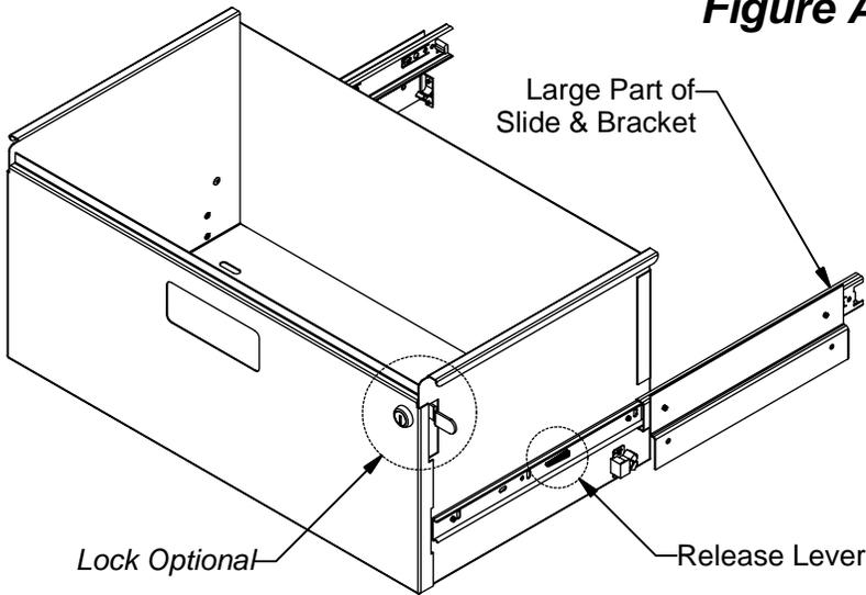
**Step 1:** Pay close attention to how Slide properly functions before disassembling to aid in reassembling later. Remove Large Part of Slide that is riveted to Bracket by engaging Release Lever to allow this part to slide off.
