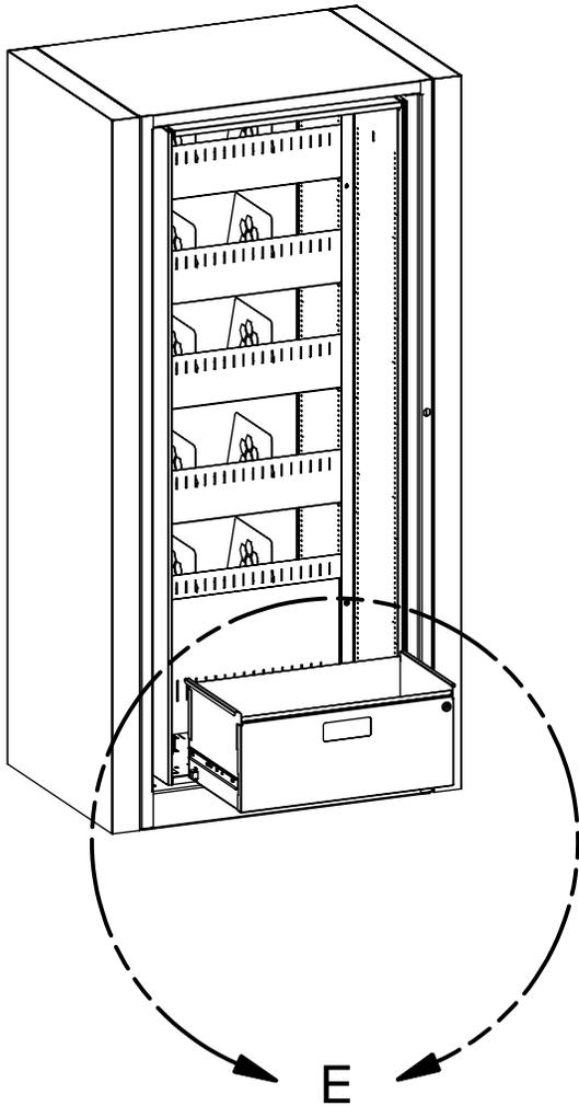
**Step 3:** Install Drawer by reassembling parts of Slide.
