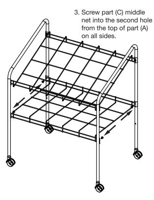
4. Screw part (B) stepped Base net into the third hole from the top of part (A) on all sides.
