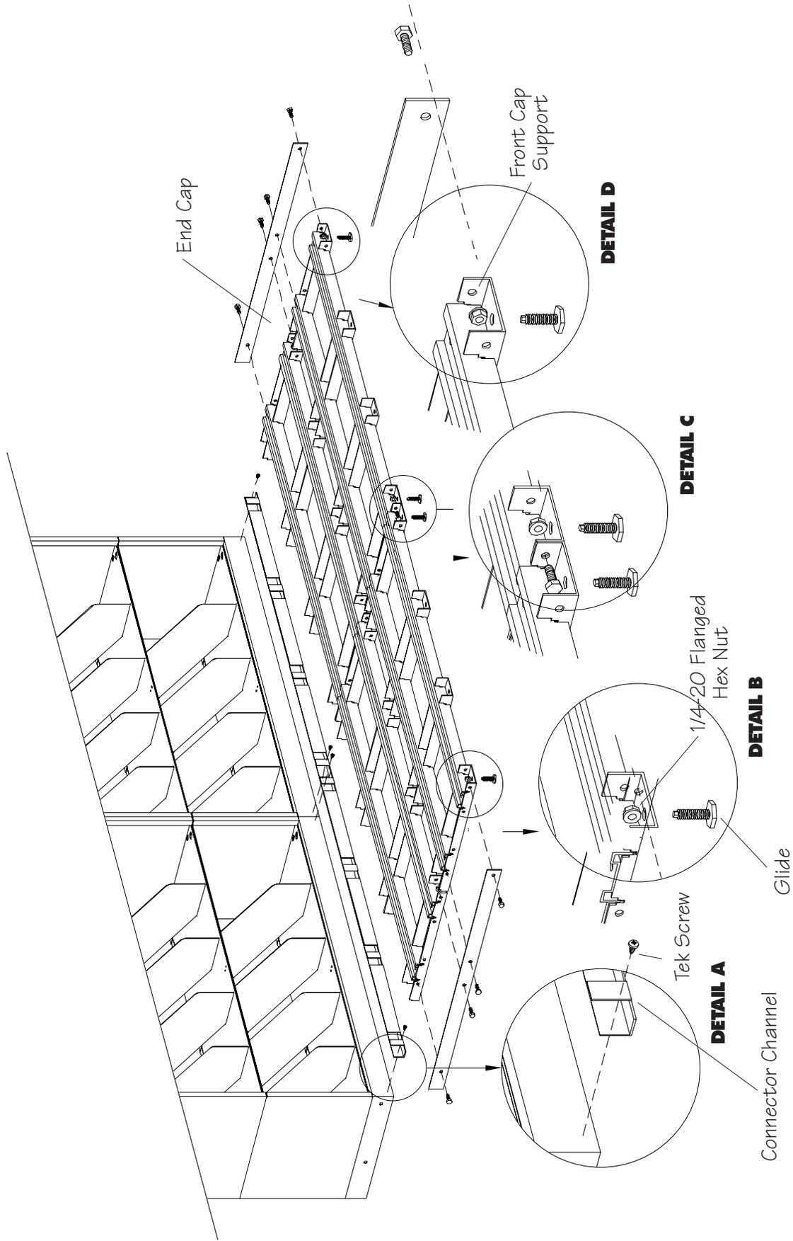
**STEP 8: LEVELING:** Determine highest point on the rail assembly. Working out from this point, level the rail by adjusting the leveling glides. **IMPORTANT!** For system to function properly all rails must be level from left-to-right, front-to-back, and rail to rail. All leveling glides must be in contact with the floor.
