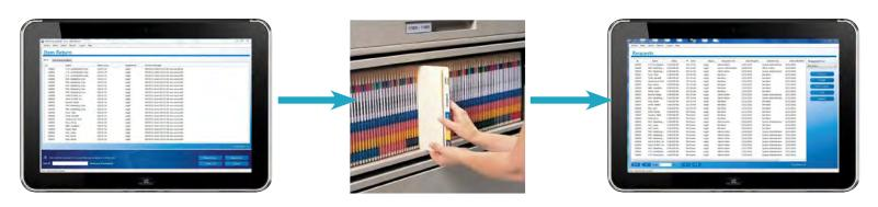
MasterTrak Essential HDSA is designed to facilitate efficient picks and put-aways from Carousels and High Density Storage Systems. Users can sort their Requests pick lists and Item Return lists by storage Zone on their tablets and move through the storage system in the most productive manner.
