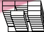
TriSlider System (T632LT8 Shown) Storage Capacity - 1,960 Lineal Filing Inches* Footprint - 32 Square Feet
