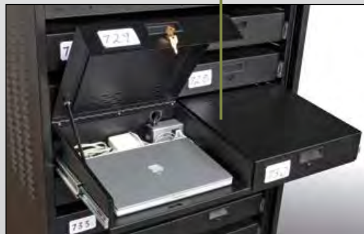
#050-00747 Secure Laptop Drawer (can accept laptops up to 14.75" x 12" x 3" high). Secure Laptop Drawers come complete with a 2-outlet power bar and has (2) private chambers with lockable lids. Note: Each lid is keyed differently to all other lids in the cabinet or cabinets unless specified. Master Keys available. Space required: 6"
