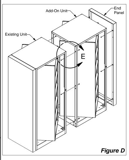
**Step 2:** Position Add-On Unit beside existing unit. It may be necessary to adjust leveling of Add-On Unit to get keyholes to align. Use six 1/4-20 x 5/8" Phillips Pan Head Machine Screws & Flanged Hex Nuts to secure the two units together as shown in *Figure D & Detail E*.
