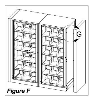
**Step 3:** Fasten six 1/4-20 x 5/8" Phillips Pan Head Machine Screws into End Panel if they aren't already there. Do not tighten them at this time though, just get them started. Insert screws of End Panel into large part of keyholes on unit & screws on End Panel should now move into lower part of keyholes. Tighten all six screws. See *Figure F & Detail G*.
