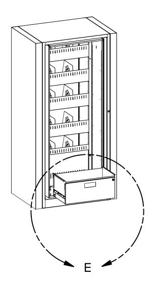
**Step 3:** Install Drawer by reassembling parts of Slide.
