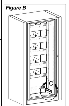
**Step 2:** Attach each Bracket with Large Part of Slide to desired location on cabinet with two #10-24 x 1/2" Type 'F' Phillips Pan Head Screws as shown in *Detail C*.
