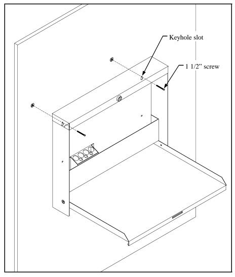
Insert 1 1/2" screw into KapToggle<sup>TM</sup> anchor. Do not tighten all the way. Mount WallWrite over these two screws and tighten.
