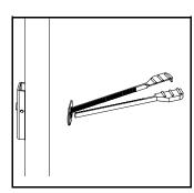
Snap off plastic straps flush with washer.
