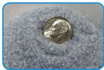
Optical media particles: <1.5mm 2 , nearly as fine as salt
