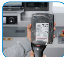
Barcode reader documents hard drives being shredded
