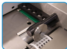
Bottom-suction air feed system
