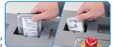
Separate feed openings for 3.5" and 2.5" drives
