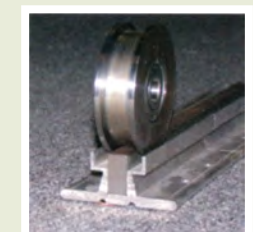
All systems have dual flange wheels to eliminate carriage derailment
